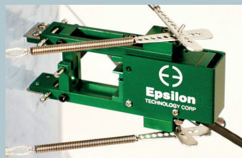
Model 3542 configured for a very large specimen diameter
