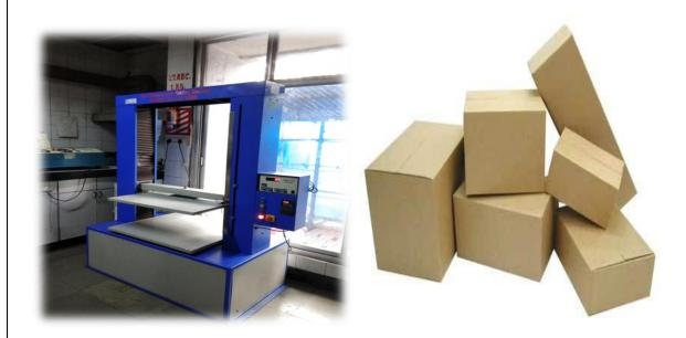
Box Compression Testing Machine is to determine the resistance of the box to vertically applied compressive loads during transit and storage. The ultimate test for determining overall quality and performance of the packages.
