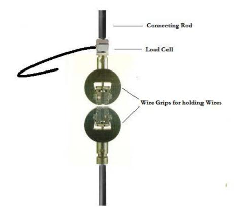
Wire Testing Kit for dia. 1.5 to 5.0 mm, consist of Vice cum wedge grips set, bare attachment set and 1 S Type load cell (Capacity upto 50 KN).
