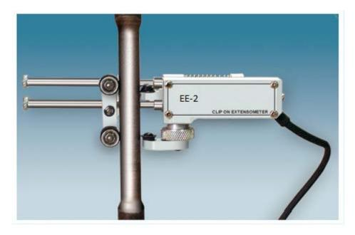
The electronic exensometer, Model EE-2 is manufactured as per IS:12872:1990 & ISO 9513:1989 in class 1 accuracy.
